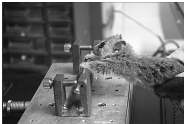
Figure 1 Picture of an individual performing a pull strength test.
